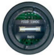
Figure 1 – 2048 Pixel Line Scan CCD Chip
