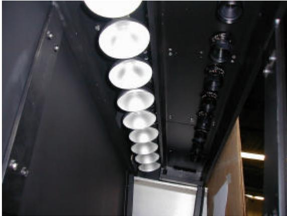
Figure 17 - Lamp Assembly containing 16 R30 Flood Lamps
