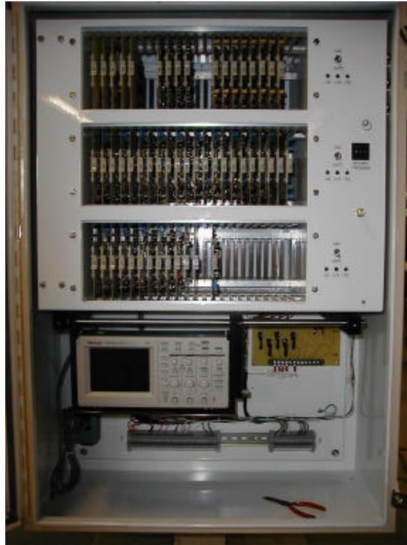
Figure 26 - low voltage DC power supplies, module racks, electronic modules, engineering workstation, oscilloscope, and miscellaneous electronics and hookups
