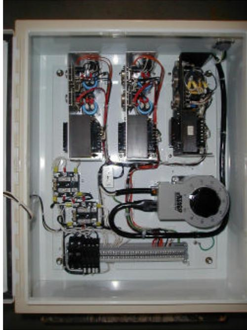
Figure 24 – Lamp Power Assembly
