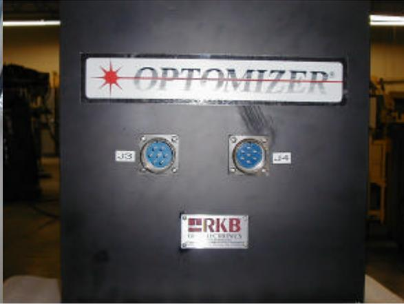
Figure 15 – J-Plug; 7 Pin power & Sensing Connections
