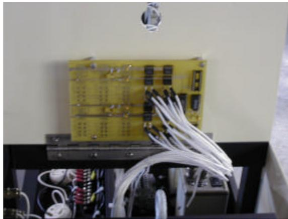
Figure 19 - Camera Sync Distribution Module
