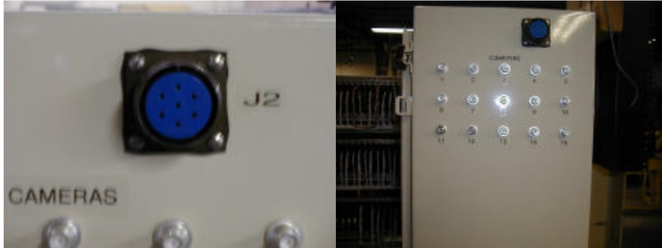
Figure 28 – J2 Plug & RG188 BNC Coax Connectors
