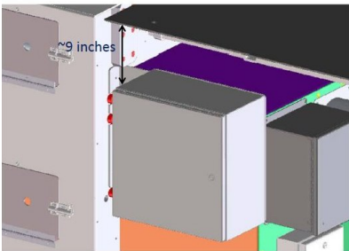
Control Box location
